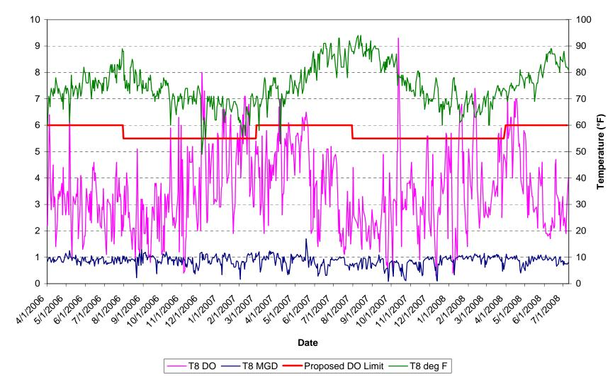
Figure 5. Tank 8 (Final Effluent) Characteristics: Flow, DO, Temperature
